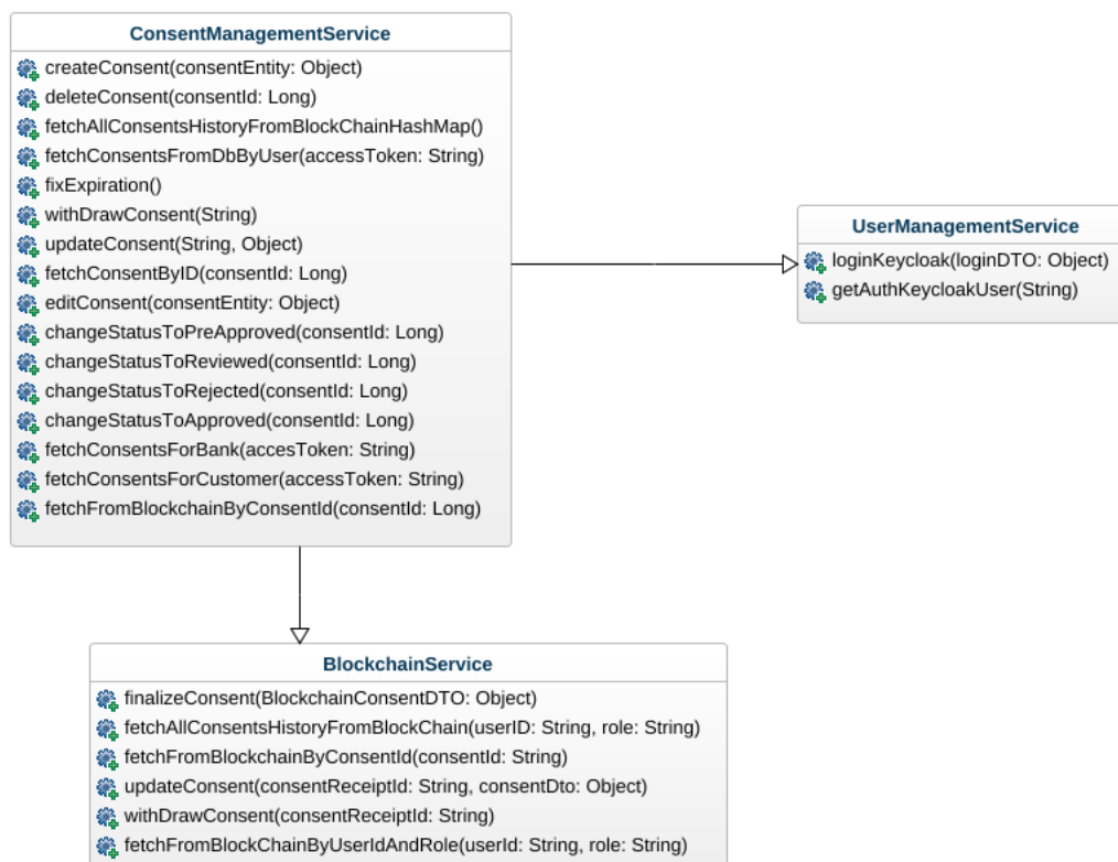
Figure 15: Consent Management System source code structure
